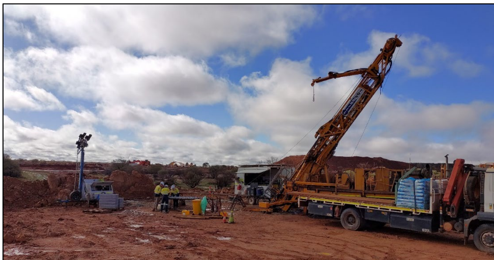
Figure 1: Topdrill diamond drill-rig drilling DGDH032 at the Never Never Gold Deposit, Dalgaranga Gold Project.
